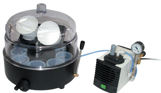
Vacuum impregnation unit
