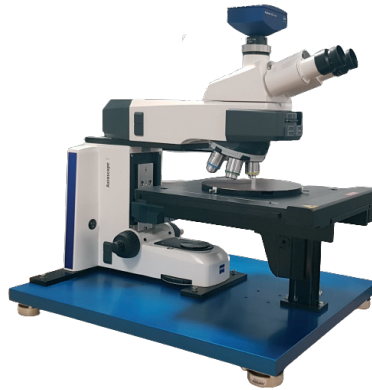
Custom build – 8" wafer microscope with automated stage and focus
