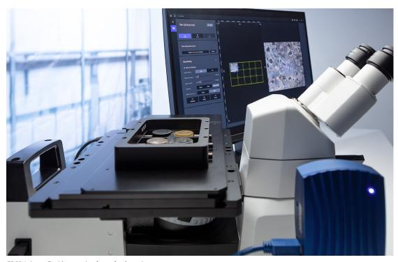
ZEISS Axiovert 7 with mounting frame for 6 specimens
