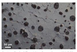
Cast Iron, Circular-Differential Interference Contrast (C-DIC) EC Epiplan 20×/0.4
