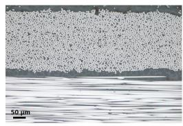
Carbon fiber reinforced polymer, EC Epiplan 20×/0.4
