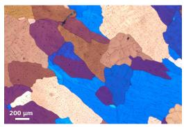
Aluminum anodized, Polarization Contrast , EC Epiplan-Neofluar 5×/0.13
