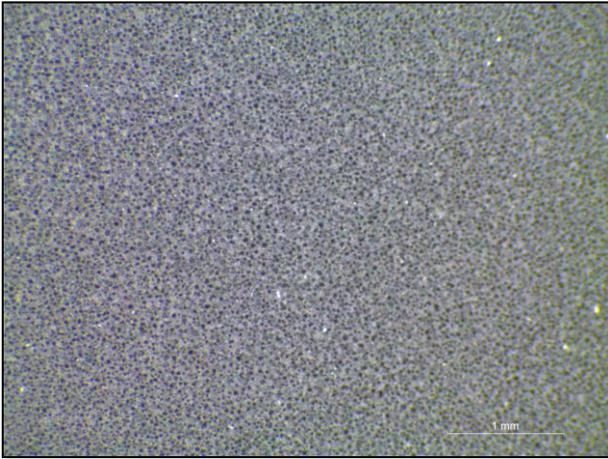
Chemicloth Stereo Microscope at 20x
