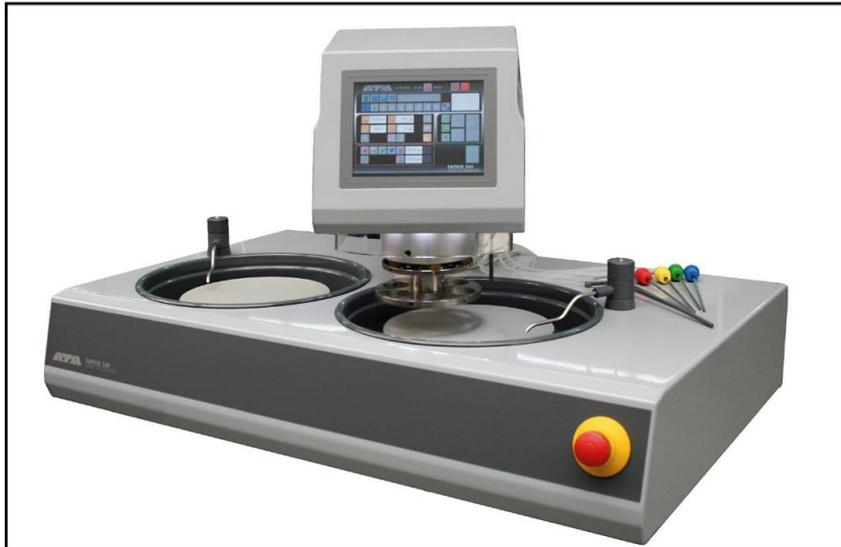
Such machines as illustrated above combine a programmable head, twin platens, and a sample holder to allow individual samples to be prepared ensure controlled & repeatable metallographic sample preparation. Controlled preparation means operator independent results, faster throughput and consistent microstructures revealed.
