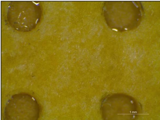
Planocloth H Stereo Microscope at 20x
