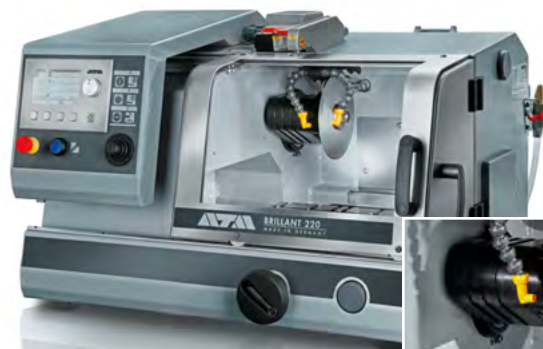
BRILLANT 220 Precision cutting and thin section preparation with Vice 6
