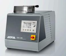
The OPAL 480 is a fully hydraulic, water cooled hot mounting press for mounting samples before polishing. The process sequence is executed automatically. The fully automatic sliding closure allows quick and easy opening/closing of the mould assembly. Mould assemblies can be exchanged quickly and without tools.
