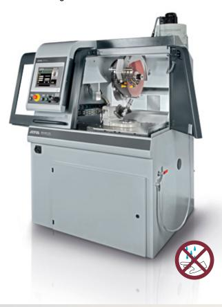
The 5-axis cutting robot Brilliant 3D has 2 additional axes (D, E-axis). This allows the specimen to be positioned and cut automatically in a single operation in nearly any position to the cutting wheel.
