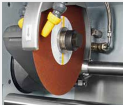
Large cut-off wheel of 254 mm / 10" with parallel moving wheel guard
