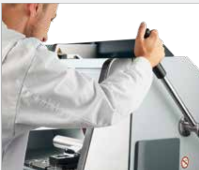
Manual Y-axis for chop cut with automatic lever brake for easiest handling
