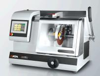
The Qcut 250 A (Brillant 240) is a compact and flexible semi-automatic abrasive cut-off machine with a 254 mm/10" cut-off wheel for workpieces or samples up to Ø 95 mm. This machine combines the benefits and speed of a manual cut-off machine with the advantages of an automatic abrasive cutter.
