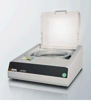
The vibratory polishing device Qpol Vibro (Saphir Vibro) is designed for the preparation of specimen surfaces practically without deformation. This preparation method is especially suited for further characterizations like EBSD (electron backscatter diffraction), nano indentation using AFM (atomic force microscopy) or micro hardness testing.
