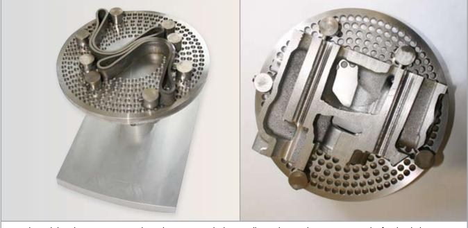
Samples with big dimensions or complicated geometries which normally need manual preparation can be fixed with the new universal sample holder for automatic grinding and polishing.
