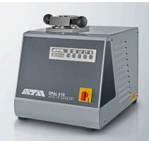
The OPAL 410 is a fully hydraulic, water cooled hot mounting press for mounting samples before polishing. The process sequence is executed automatically. Mould assemblies can be exchanged quickly and without tools.
