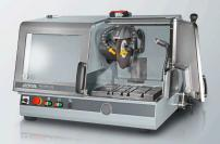
The BRILLANT 230 is a wet abrasive cut-off machine with fine dynamic, manual wheel movement into samples up to Ø 110 mm. The spacious cutting chamber allows various clamping variations. The solid aluminium design of the cutting machine comes with openings on the right and left hand side for cutting continuous long parts.
