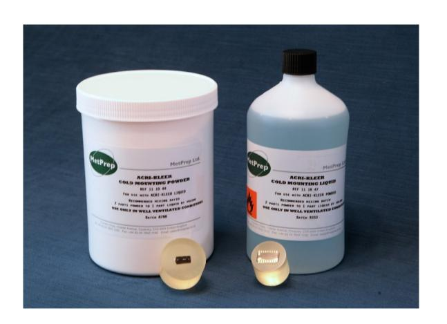
MetPrep's most transparent powder / liquid acrylic mounting system without using a pressure chamber. Ideal for many applications where seeing into the mounted sample is required. It is particularly popular for PCB micro-sectioning and microelectronic applications. Combines excellent visibility with good edge retention for an acrylic system.
