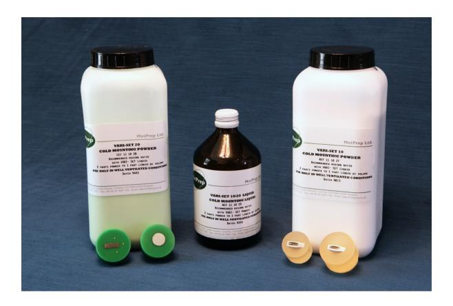
MetPrep's revolutionary powder / liquid mounting system offers a soft clear or hard filled option. The hard filled VARI-SET 20 offers excellent edge retention for a quick setting acrylic and the soft clear VARI-SET 10 is ideal when some transparency is required.
