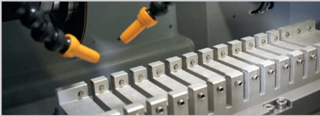
Cutting device for fish ear bones
