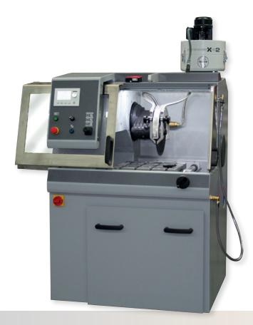
The universal wet-abrasive cut-off machine BRILLANT 265 with automatic travel and cut-off allows precise, soft touch cutting with 2 axes in arbitrary directions (Y/X axis) and can be equipped with an automatic or manual Z-axis for parallel serial-cuts (option).
